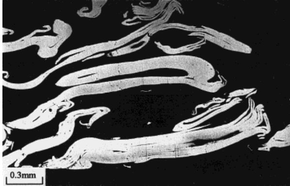
Figure 4 OM photograph for the distribution of the Al flakes in the gate.
